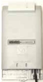
4. Separate the router face plate from the mid-plate by unclipping it. Remove the black protective rubber dust cap from the mid-plate fibre receptacle and the dust cap from the end of the cable and slide the mid-plate down until it locks into place.
